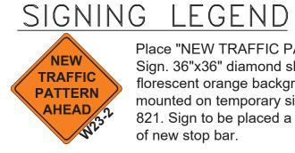
Place "NEW TRAFFIC PATTERN AHEAD" W23-2 Sign. 36"x36" diamond shape warning sign with florescent orange background with black letters, mounted on temporary sign support. See detail TM 821. Sign to be placed a minimum of 250 feet ahead of new stop bar. NOTES
