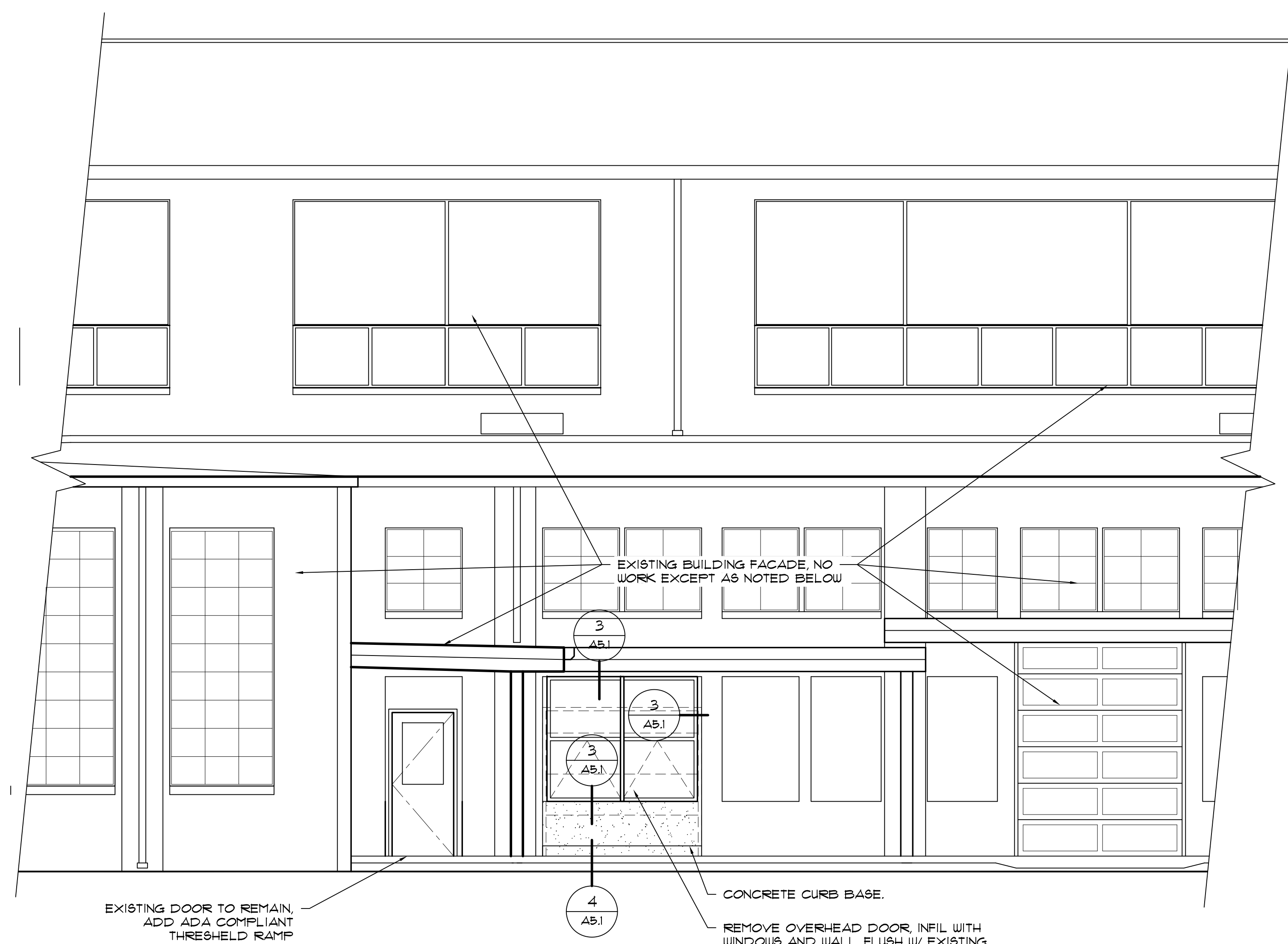
1 PARTIAL EAST ELEVATION SCALE 1/4" = 1'-0"
